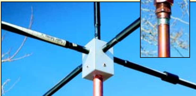
Close-up views of the antenna and the coupling between the two halves of the base shaft.
